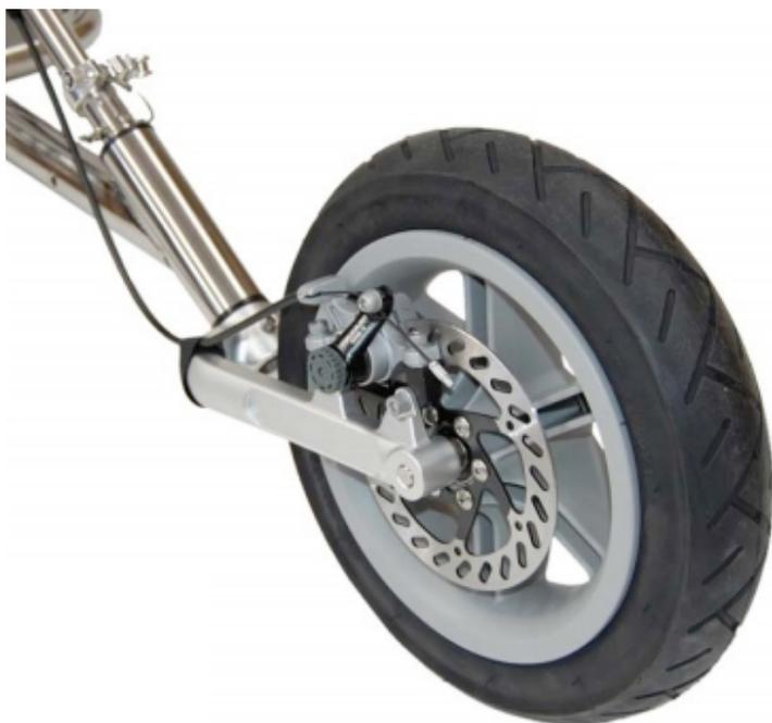
The Blokart Disc Brake is a piece of high precision equipment with fine tolerance. Any sand or grit from beach sailing may affect its performance.
