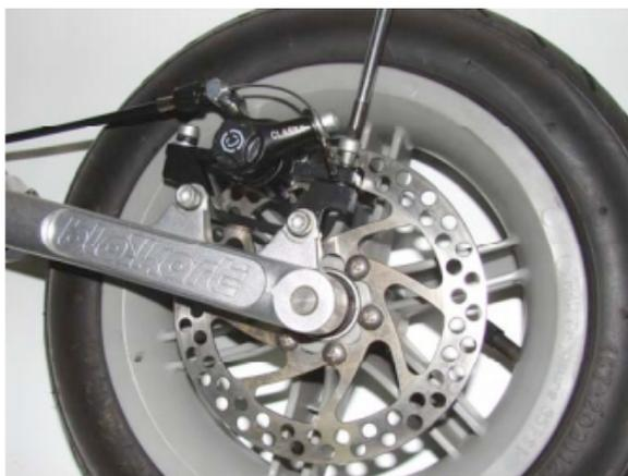
Remove the calliper mounting screws from the calliper mounting block. Loosen the brake pads on the calliper by rotating the adjusters either side and align the mounting block with the holes on the fork.
