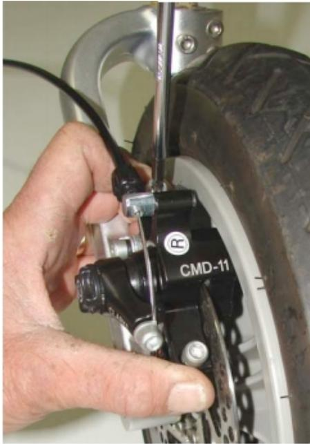
Align the calliper so the rotor is centered in the slot of the alloy casting and secure the alignment screws.
