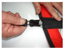
3. Double-up the bungee by pulling the batten cap, locating it on the batten end for a snug fit.
